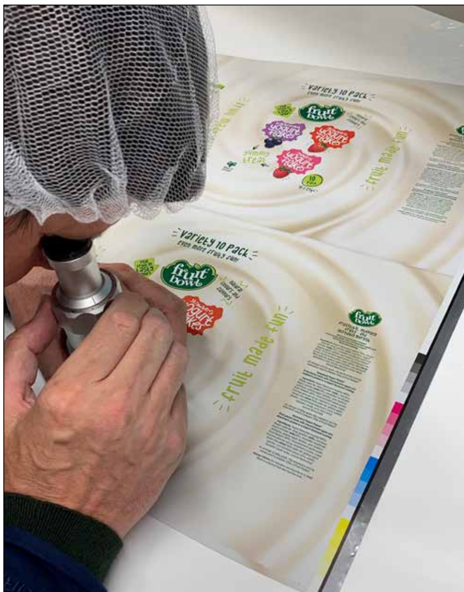
Fruit Bowl Yogurt Flakes, printed with Project Blue and its hybrid screening platform, depicts enhanced dot patterns, flat solid colors and sharper text edges than conventional HD flexo print. This package is 5-color: CMYK plus white.
